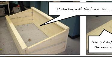
Using 2 6-foot boards in 2x12 for the rear and 2x8 for the front
