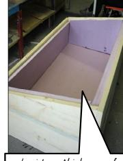
Inside, a thickness of polyurethane insulation is added
